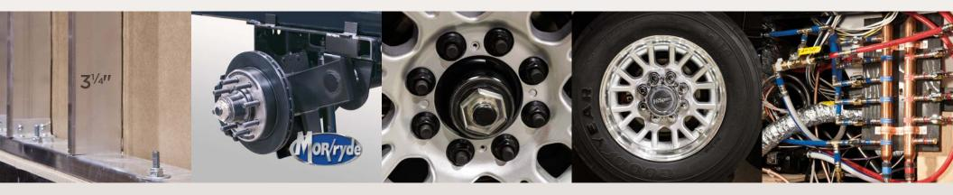
Our 3 1/4" walls are the thickest in the industry, giving you maximum insulation from noise and weather. The exclusive foam core vapor barrier eliminates condensation.
