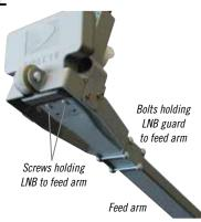
6. Slide the LNB guard up the feed arm and over the LNB. The front of the LNB guard should be ~½" in front of the LNB and should not be touching the LNB. Install the four bolts through the four holes in the LNB guard. Thread a nut onto each bolt, and tighten.
