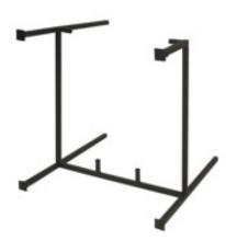
6. Attach the horizontal (8) inserting the studs from the legs into the horizontal. The studs in the middle of the horizontal should face down, and the hooks for the stairs should now point toward you with the opening facing up.
