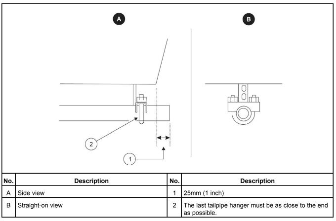
FIGURE 6. TERMINATING THE EXHAUST TAILPIPE
