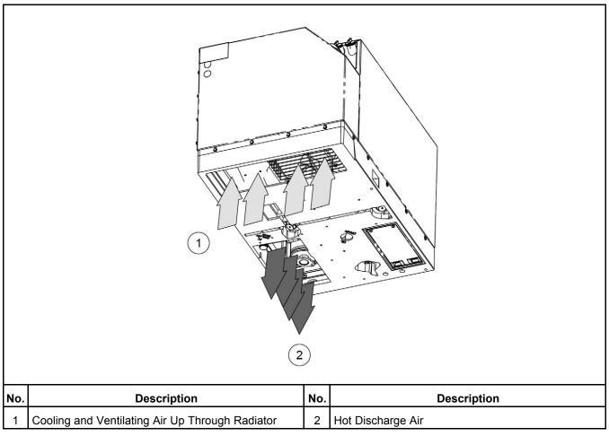
FIGURE 2. COOLING, VENTILATION, AND COMBUSTION AIR FLOWS
