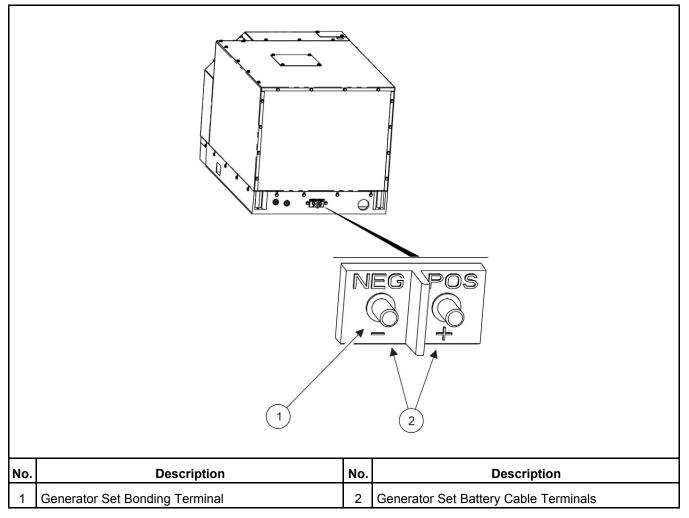
FIGURE 15. BATTERY CABLE CONNECTIONS
