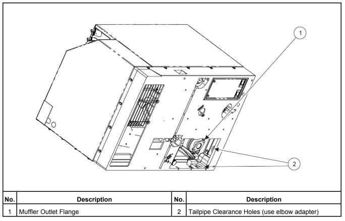
FIGURE 3. TAILPIPE INSTALLATION
