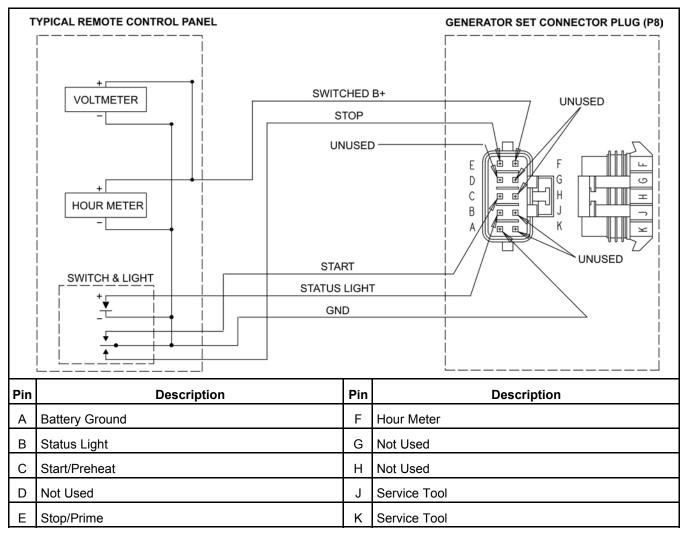
FIGURE 12. REMOTE CONTROL CONNECTOR PLUG AND TYPICAL CONNECTIONS
