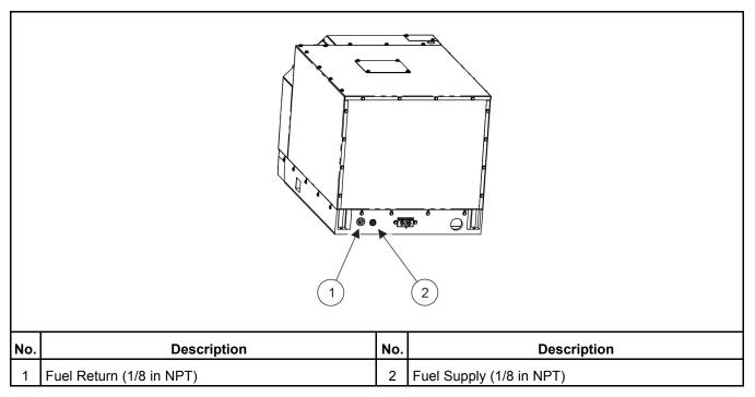
FIGURE 8. FUEL CONNECTIONS
