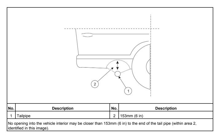
FIGURE 5. MINIMUM DISTANCES TO OPENINGS
