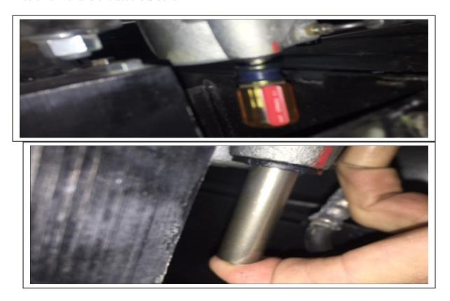
**Step 5:** Apply Red Loctite to the new Caliper Guide Bolt.
