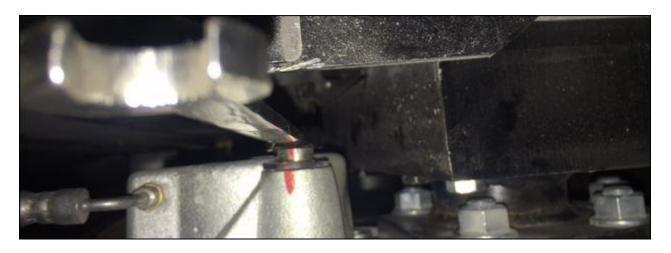
**Step 3:** Insert a small screwdriver into the Sleeve, apply a slight torque on the screwdriver and extract the Sleeve.
