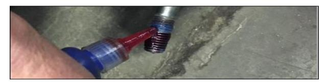
**Step 6**: Using ratchet wrench, reinstall the Caliper Guide Bolt.
