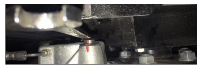
**Step 7:** Using torque wrench, tighten the Caliper Guide Bolt to 45 ft-lbs.
