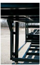
Pinless hydraulic jacks are mounted at a 5-degree angle for maximum stability.
