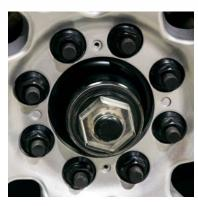
Commercial E-Z Lube® hubs surrounded by 8 large 5/8" stud bolts and standard automotive disc brakes round out the safety features of every DRV unit.
